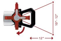
Wide Spray - wide angle / large orifice opening. Ideal for large areas and a high working speed.
