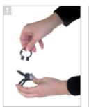
Place the TR<sup>2</sup> tip holder onto the tip guard and close it.
